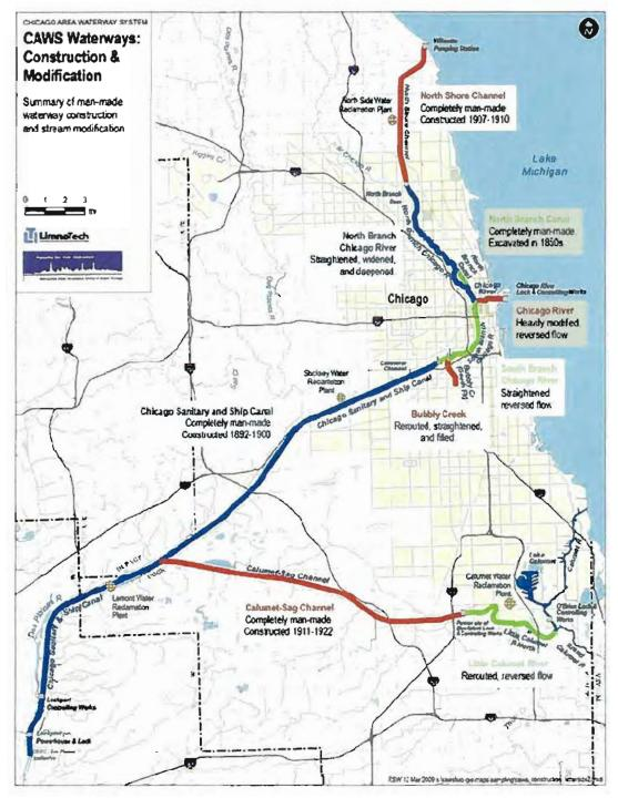
Figure 2-1: Construction and Modification History of the CAWS
